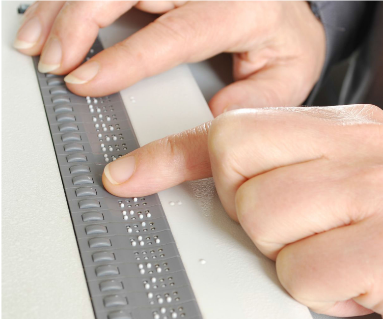
Fig. 11.1 A screen reader captures text on the screen and displays it on a Braille device
