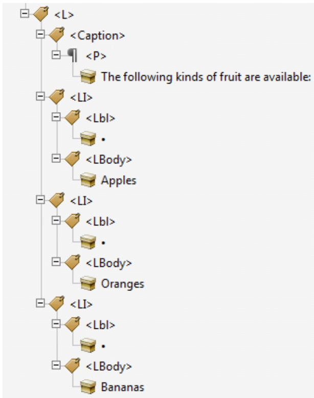
Fig. 10.6 Representation of an accessible list in the structure tree
