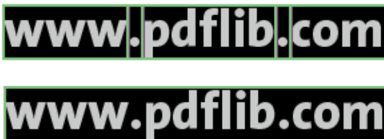
Fig. 6.5 The default setting punctuationbreaks=true will separate the parts of URLs (top), while punctuationbreaks=false will keep the parts together (bottom).
