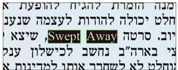
TET reorders the visual mixture of right-to-left and left-to-right text to create proper logical text output.
