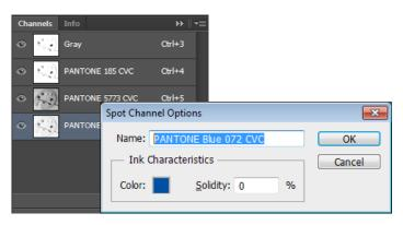
Photoshop displays spot color channels of extracted TIFF images in the Channels window (left). Double-clicking one of the icons reveals the corresponding alternate color (right).
